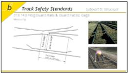
**Key Message:** The critical area where guard check gage must be measured is at the actual point of frog. Inspectors must also consider any unusual wear that may exist at the actual frog point and position the track gauge or other measuring device accordingly. It is important to also include rail crossing (diamond) frogs when considering these measurements.
