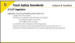
**Key Message:** Inspectors must be aware that live and dead growth, drift, tumbleweeds, debris, etc., can constitute fire hazards to timber bridges, trestles, wooden box culverts, and other track-carrying structures. Although all signals are important, the visibility of certain signals must be closely observed: i.e., block signals, interlocking signals, speed signs (or other signs affecting the movement of trains), close clearance signs, whistle posts, and mileposts.
