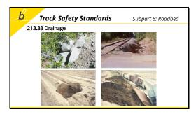
**Key Message:** One of the most essential elements of track maintenance is a comprehensive drainage system. Drainage facilities (bridges, trestles, or culverts) should be given careful detailed consideration during inspections. Openings under the track are used to channel and divert water from one side of the roadbed to the other.
