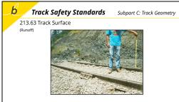
**Key Message:** Illustration of large runoff. String is held level using string bubble and distance between string and rail is measured 31 feet away from the high track.
